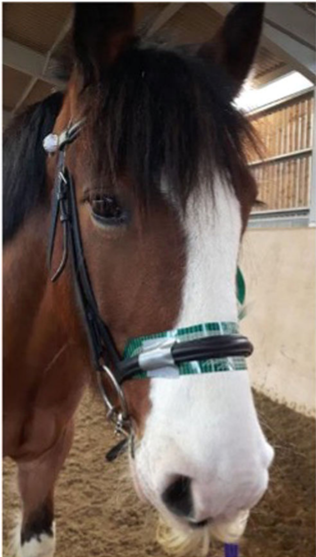
Fig. 4. Fitting of the pressure sensor mat under the noseband.
